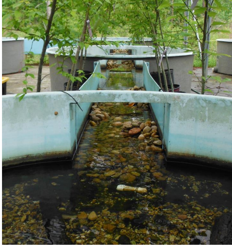
Figure 1. Picture of upstream portion of heterogeneous mesocosm treatment with larger substrate, shallow water, increased canopy cover and current velocity.
