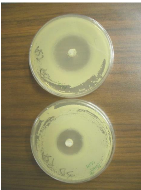
Figure 3. ZOI test results for norfloxacin (top) and NOR-treated fluoromica (bottom)
