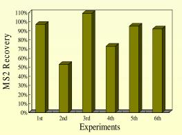
The hollow fiber filter was not blocked with calf serum in Experiments 2 and 4 resulting in lower MS2 recovery rates.
