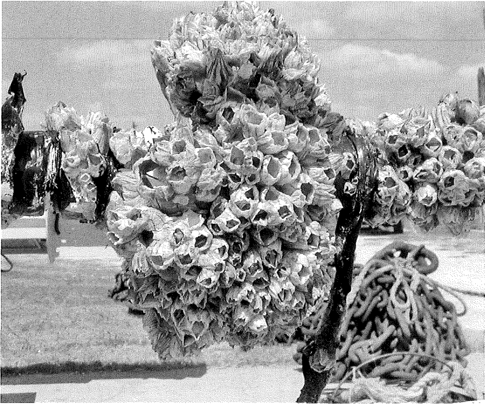
Fig. 3. Barnacle encrusted Aanderaa DCS 3900 sensor recovered from site R after a 6-mo deployment. The velocity data were acceptable in spite of this level of fouling.
