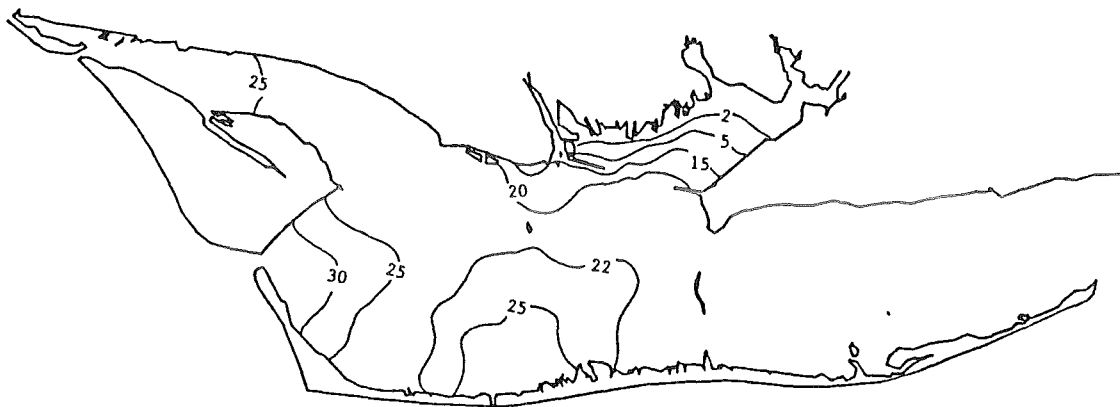
Figure 21. Salinity Contours of the Lower Layer at the High Tide - With Horizontal Density Gradient Terms.
