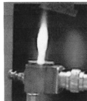
FIG. 2. A typical picture of the microwave induced plasma operating with argon carrier gas.
