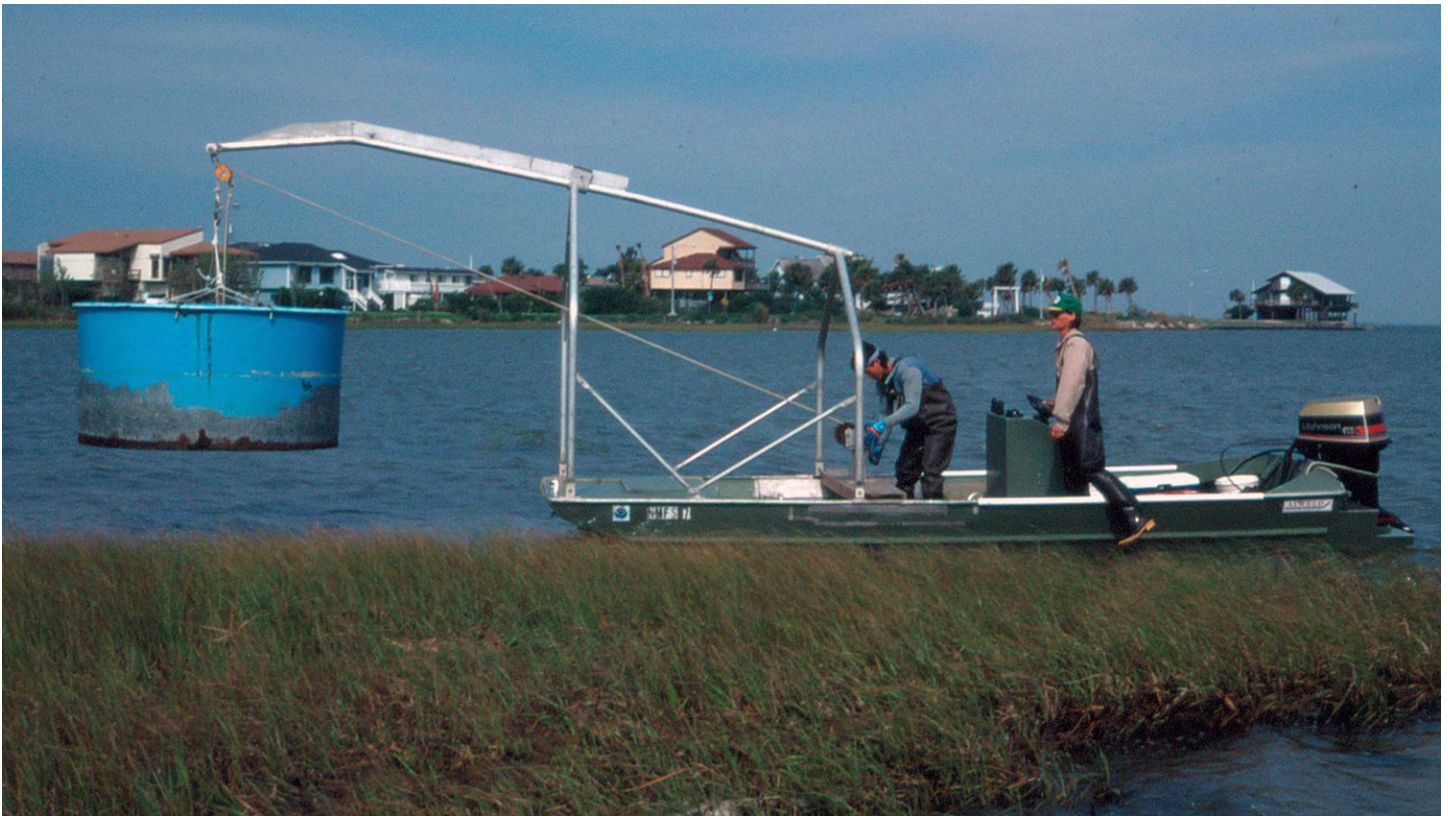
FIGURE 3. Drop sampler used to collect nekton in Gulf of Mexico salt marshes
