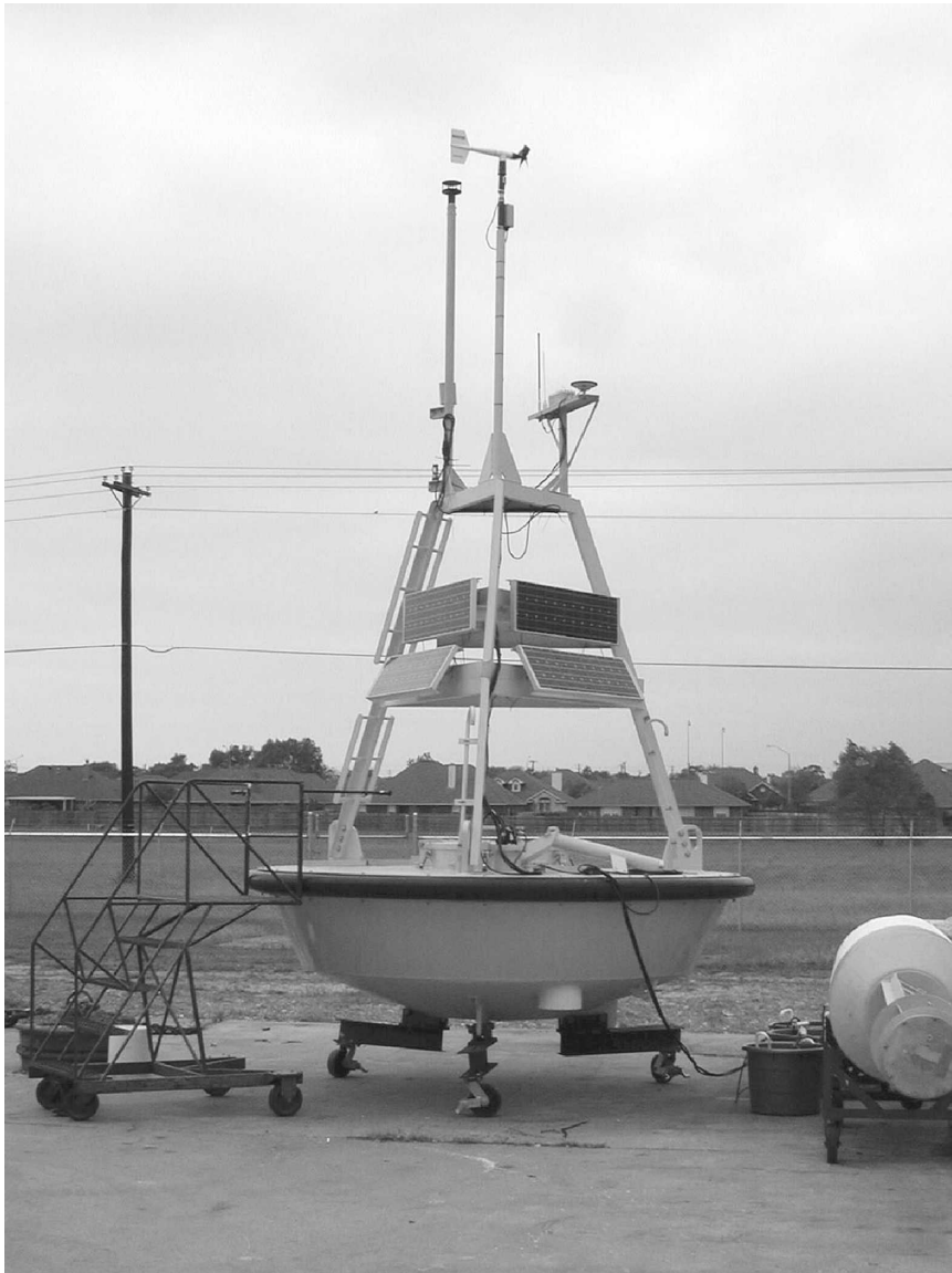
Fig. 2. Buoy during burn-in test at GERG. The Gill WindSonic is on the mast to the left and the R. M. Young is on the mast to the right.
