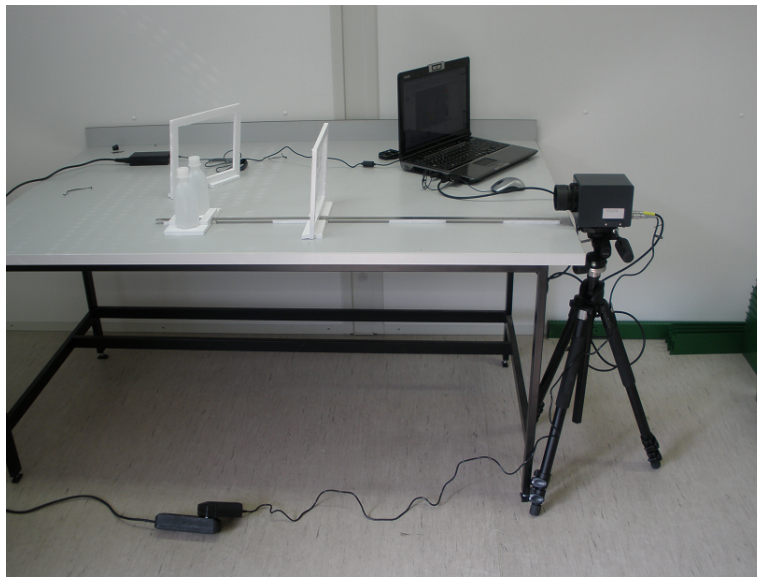
Figure 3.1: General setup of infrared thermography calibration measurement experiment.
