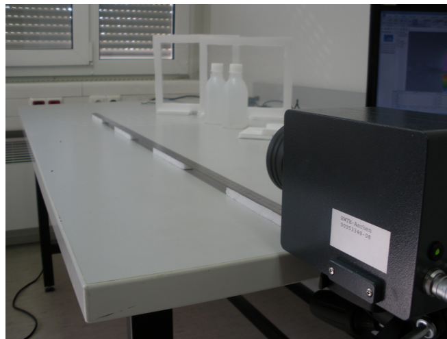
Figure 3.2: IR camera and guide-ruler settings for IR thermography calibration experiments.
