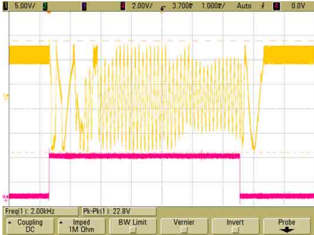
Figure 4.4: Audio module output of an entire chirp
