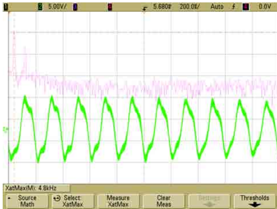
Figure 4.6: Audio module output and FFT with 100% duty cycle
