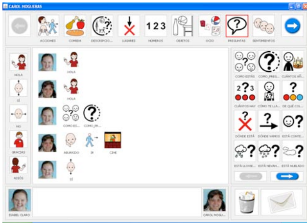
Figure 2. Dialogue window allows users to communicate by means of exchanging pictograms. The user interface is made up by five key elements. The top row contains the categories in which pictograms are classified. The left column contains the most frequent pictograms in a conversation. The right matrix contains the pictograms that belong to the active category. The central part contains the actual conversation. Finally, the bottom row contains the pictogram input space to write a message.
