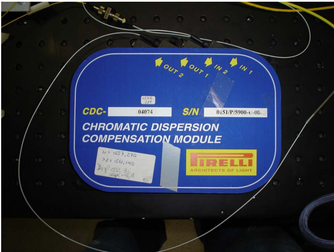
Fig. 5.23 Chromatic Dispersion Module Pirelli
