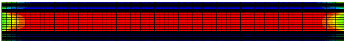
Fig. 5.9 Picture of the whole FEM specimen to illustrate the range of the edge effects.
