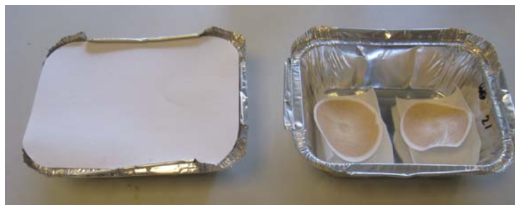
Figure 3. Aluminium support used for filter manipulation in the oven and desiccator.
