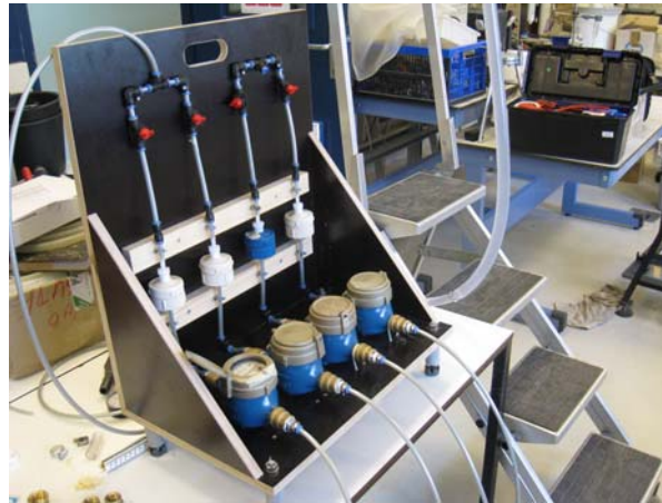
Figure 6.1. Installation of the MuPFiS at the TU Delft's water laboratory
