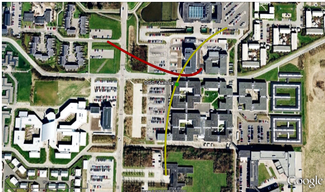
Figure 3.20: Google Earth plot of samples in Figure 3.19. The green sample represents the actual position of the antenna. Yellow: fixes from samples with induced distance bias towards North. Red: fixes from samples with induced distance bias towards East. All samples are grabbed to the ground.
