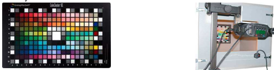
Figure 3. CCDC chart placed inside the light booth. The tele-spectra-colorimeter used is also shown.
