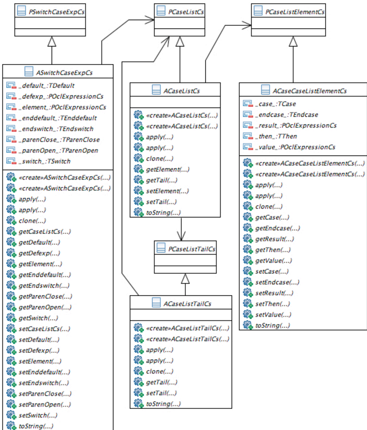
Figure 14.3: Complete SableCC-Ext generated classes for switch-case productions
