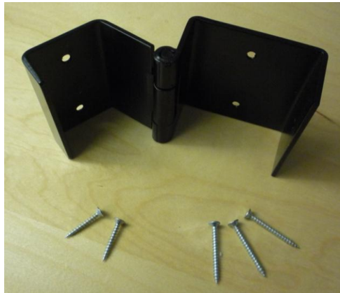
Figure 32.- Links between base frame and backrest
