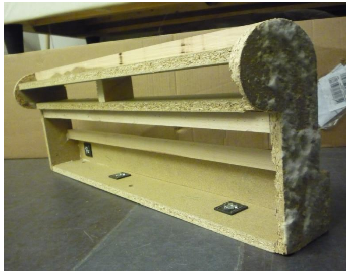
Figure 34.- Internal armrest structure 1
