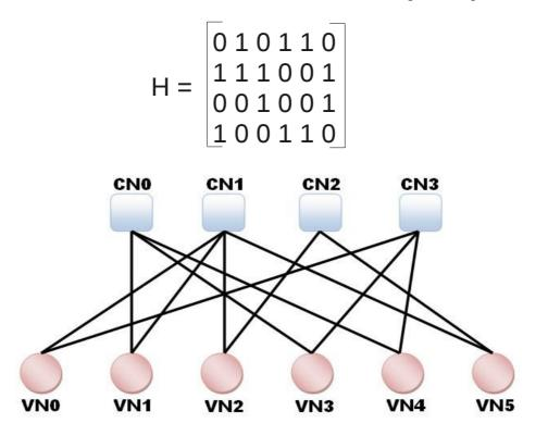
How it's shown, there are two groups of nodes; 4 CN nodes, as the number of rows and 6 VNs as the number of columns. And there's a connection between nodes CN and VN depending on the H matrix: CN0, representing the first row, is connected to VN1, VN3 and VN4 because in those
