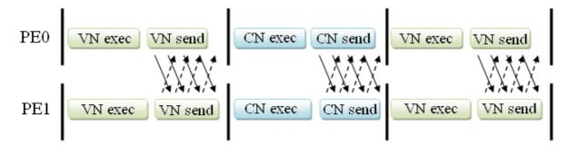
Each time slot, the ASIP, alternately, performs the node operation (Variable or Check) as a calculation phase and then sends all the messages created through its data interfaces. The associated PHAL gets these messages and delivers it into the network.
