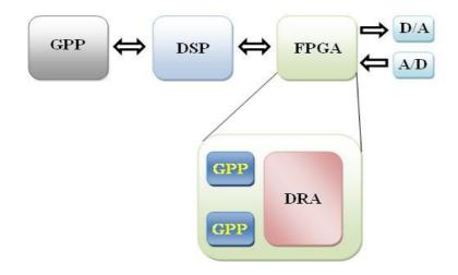
A more general scenario considers a network of mixed devices with static and reconfigurable part, as in the figure above. The designer benefits from the joint computing capacity of all elements. From here and beyond, we will use the term Processing Element (PE) for the static part and Dynamic Reconfigurable Area (DRA) for the reconfigurable one.
