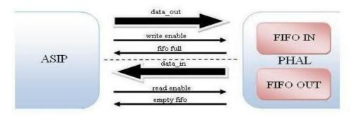
If the ASIP needs to send data, looking the fifo full control signal from the PHAL output fifo for that it doesn't get filled, it set the write enable and put the word in the output 32-bit bus. Meanwhile, when the PHAL input fifo contains some data word for the ASIP, it puts low the empty fifo control signal; in that manner, the ASIP will know that there's some data to adquire. By settin the read enable control signal it will get the word to be stored in its memory.
