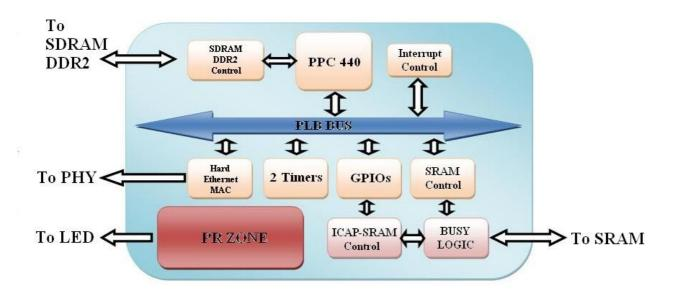
The figure shows the processor architecture: PLB bus is used to access the hard-coded Ethernet MAC controller and the external GPIO ports interfacing the reconfiguration control logic and the SRAM memory (where bitstreams will be saved).
