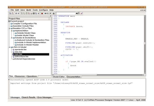
The parts, in which the code must be divided, are the main one, the instruction one and the operands and misc parts. Every section must contain some specific fields where to describe instructions and hardware resources, pipelined architecture and automatic executing instructions.
