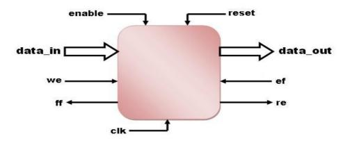
Generally, monitoring the empty fifo signal (ef), the outside agent can realice when information data is stored, put the read enable input to '1' and start catching words, one for each clock period. Every time that the read enable is put to '1' the data is thrown out and borrowed from the internal registers. When, finally, the fifo will not have more words, the empty fifo will be put to '0'.
