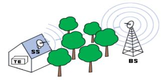
The Base Station represents the gateway allowing all the users connection to the WiMAX network: it provides coverage to all the Subscriber Stations in their area of influence and manages the traffic to and from these. The Terminal Equipment (e.g., a personal computer) is connected to the Subscriber Station to deliver it via packet traffic to the Base Station that will care to send it to the final recipient.
