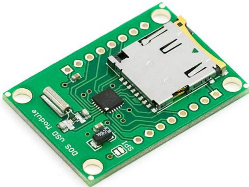
Picture 11 – MicroSD Socket with USB/FAT16 interface included.
