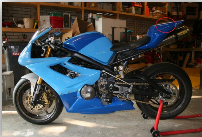
Picture 1 : Best location for TT Race Data Logger
