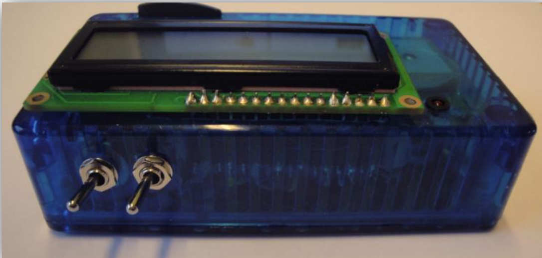
Picture 6: Two switches for manage the power supply.
