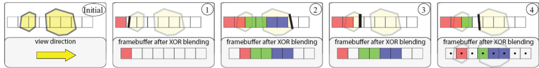
Figure 1.5: Solid Voxelization for a column in the slicemap. To simplify the illustration, only one framebuffer with two bit color channels is shown. Left: The scene, consisting of two watertight objects, is voxelized in the column along the view direction. 1-4): During rendering, fragments can arrive in an arbitrary order. For each fragment, a bitmask (upper row) is computed in the shader which indicates all voxels that lie in front of the current fragment. This mask is accumulated in the framebuffer (bottom, initialized at zero) using a XOR operation. Once the rendering is complete (4), the framebuffer contains a center sampled solid voxelization in a grid shifted by half a voxel.
