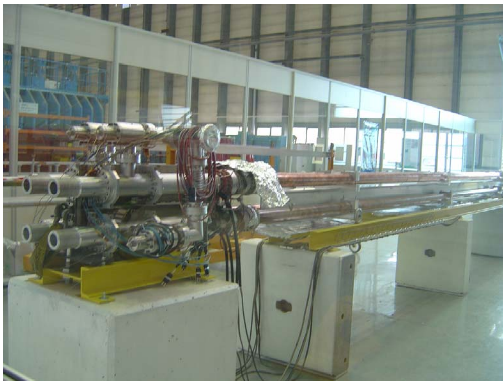
Figure 8.3. 4 LSS chambers waiting on the assembling bench to be coated
