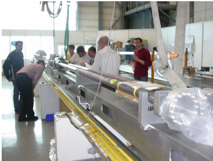
Figure 9.20. Test of the Lifting Assembly with the TAN chamber
