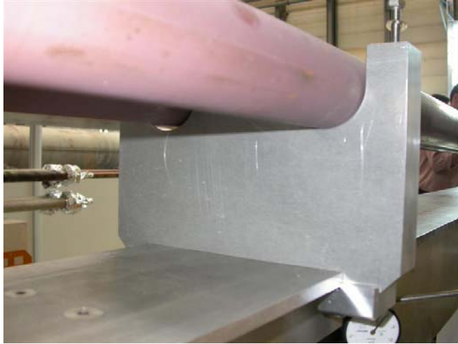
Figure 9.21. Dial gauge underneath the beamtube support
