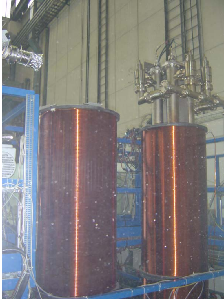
Figure 8.2. The two solenoid units. The right one with four LSS chambers being coated
