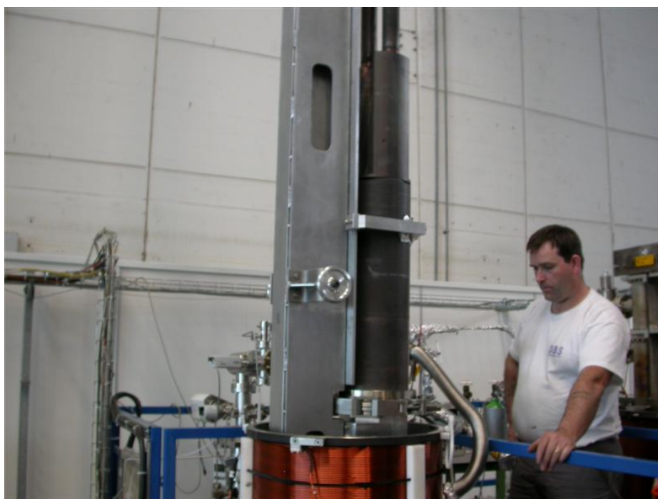
Figure 9.25. Introduction of the Assembly into the solenoid
