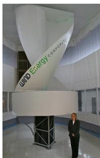
Figure 4.1.10. Helical Blade Scoop wind turbine prototype from the Wind Energy Corporation called HEB.
