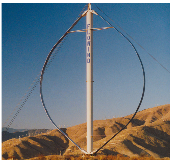
Figure 4.1.2. A 2 blades Darrieus wind turbine of the former American Flowind company.
