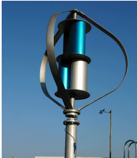
Figure 4.1.3. A Darrieus with a Savonius wind turbine to enable self-starting and rotor speed regulation.
