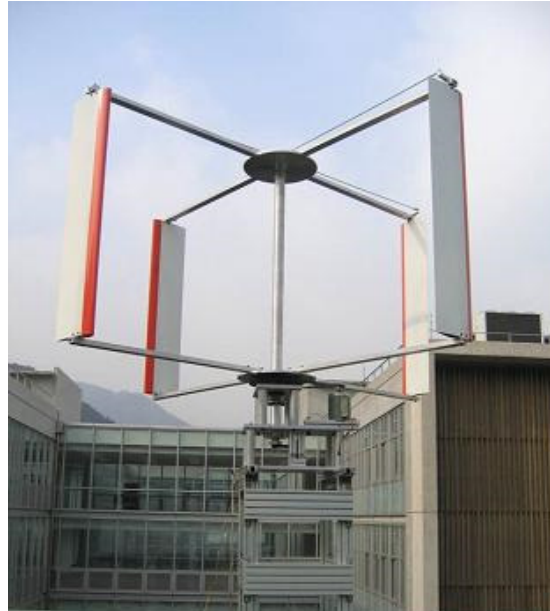
Figure 4.1.5. Small H-rotor Darrieus Cycloturbine with 2 m diameter in a top of a building [4]
