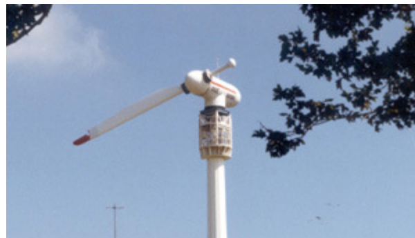
Figure 4.1.13. NASA Mod-0 research wind turbine at Plum Brook Station near Sandusky, Ohio tested a one-bladed rotor configuration, Photo by NASA Glenn Research Center.
