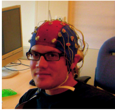
Figure 2.11: A practical way to record EEG is to place the electrodes on a helmet. Picture taken in Philips Research laboratories.
