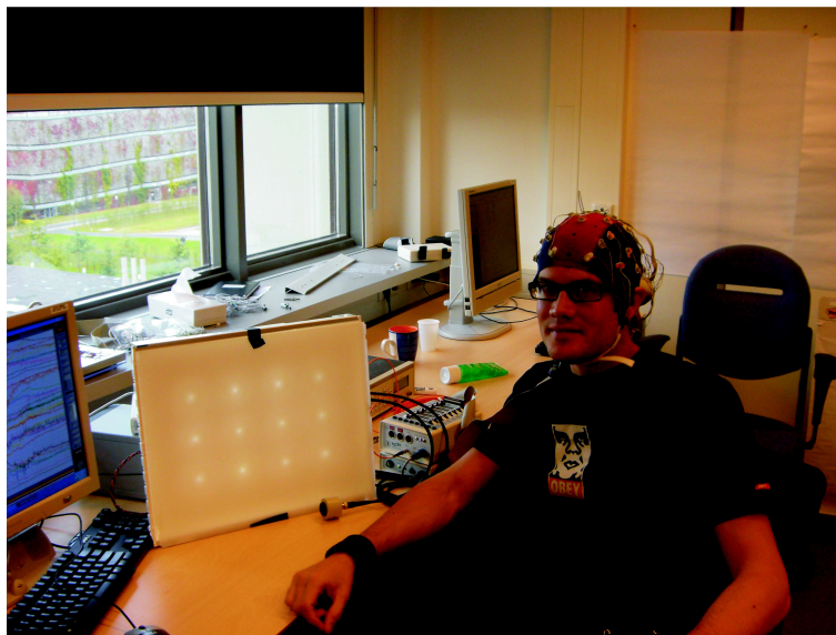
Figure 4.3: The complete setup including the cap with the 32 electrodes, the AD-box, USB2 converter and PC used for recording the EEG signals of the subject S1.
