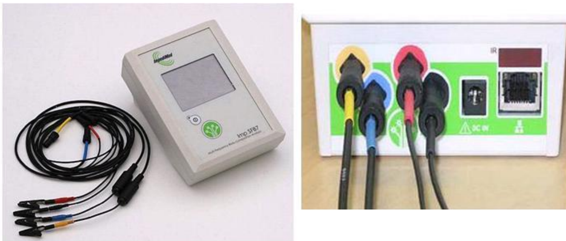
Figure 3.1 The Imp SFB7 is a 4-Electrode EBI spectrometer and back connection for the 4E-Electrodes
