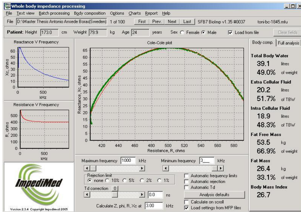
Figure 3.3 The Impedimed BioImp applications displaying whole body bioimpedance data from the Impedimed Imp SFB7 device.
