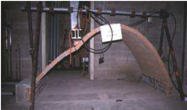
Figure 3.26: Global deformation (Valluzzi et al. 2001)
