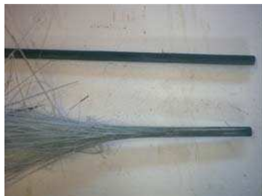
Rupture of GFRP bars (glass fiber)
