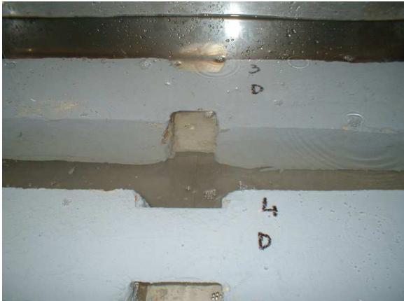
Figures 3.42: Specimens in the climatic chamber subjected to Freeze-Thaw Cycling (Desiderio and Feo, 2005).
