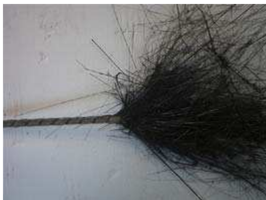
Rupture of CFRP bars (carbon fiber)
