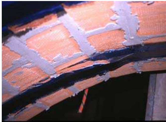
Figure 3.29: Detachment of Fibers (Valluzzi et al 2001)
