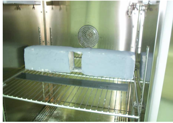
Figure 3.43: Specimens in the climatic chamber subjected to UV exposure (Desiderio and Feo, 2005).
