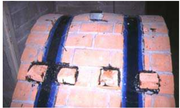
Figure 3.27: Effect of excessive confinement (Valluzzi et al. 2001)
