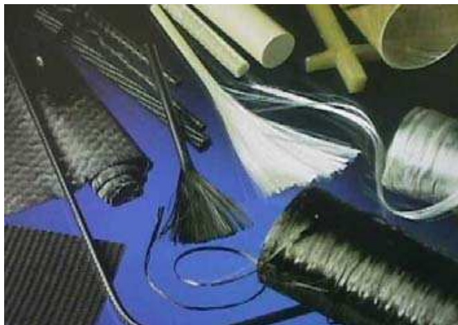
Figure 2. 30: Different FRP materials (CNR-DT 200/2004)
