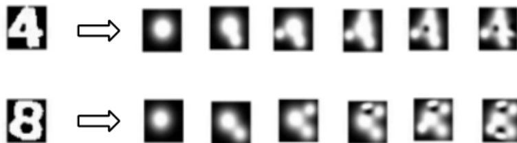
Figure 2.1: Example of image reconstruction using the MP algorithm with few atoms.
