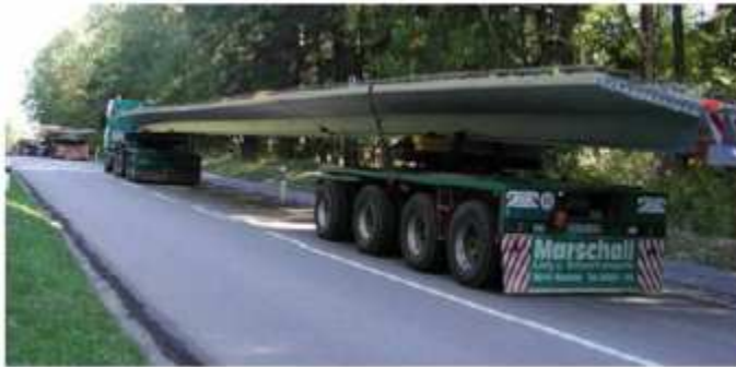
Fig. 13.8. Transport of the VFT-WIB girders from the concrete plant to the construction site
