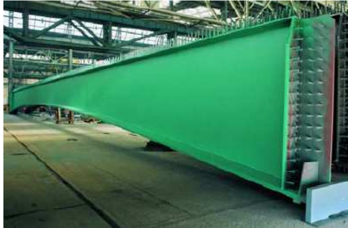
Fig. 5.1. Steel girder in manufacturing site.
