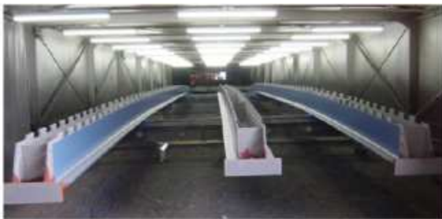
Fig. 13.6. Rolled girders after cutting and coating in the shop
