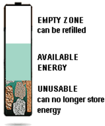
Fig. 1.2. Three imaginary sections of a battery consisting of available energy, empty zone and unusable zone [6]
