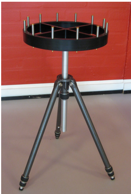
Figure 5.25: Circular array with radius of 11.9 cm and 12 microphones. Prototype implemented by Brüel & Kjær.
