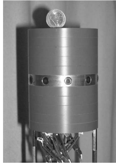
Figure 5.5: Ten-sensor circular array mounted into a rigid cylindrical baffle of length of 11.3 cm and radius of 4 cm. Picture taken from [15].
