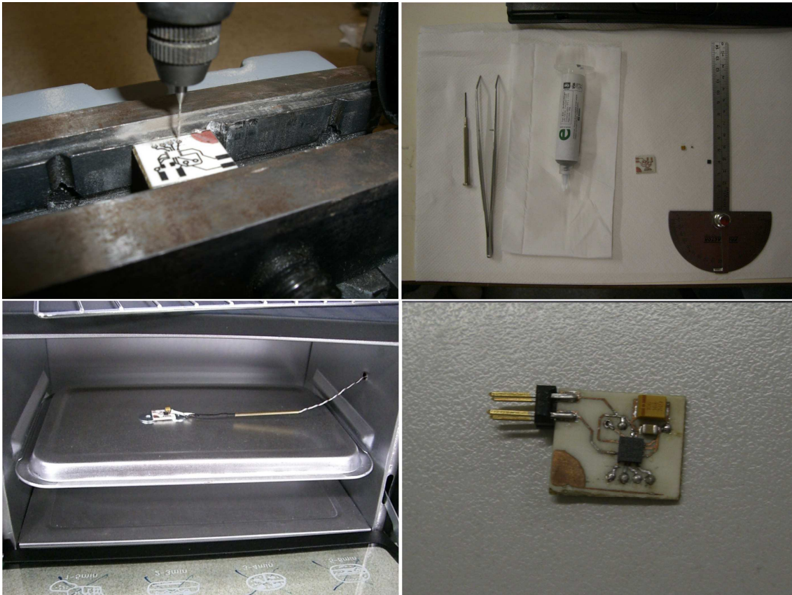
Fig. 4.8 Board in the drilling platform, with solder paste, inside the oven and the final result
