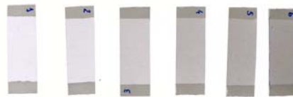
Figure 4.8: Samples with silver contact electrodes for resistance measurements.
