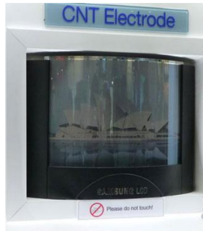
Figure 6.12: First TV screen using CNT material as transparent electrode.
