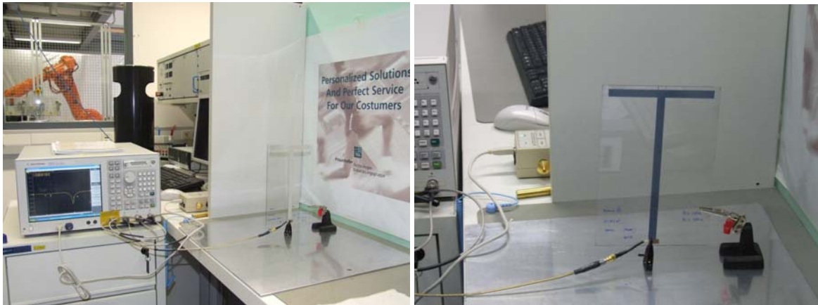
Figure 6.6: Illustration of the test routine to measure the reflection coefficient (S11) of the antenna.
