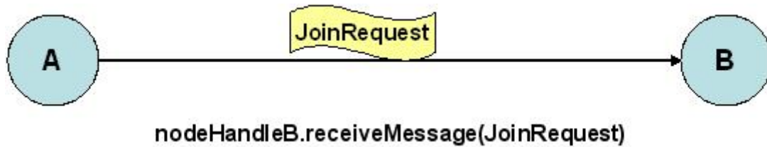
Fig 2.4 Sending directly a JoinRequest message from A to B.
