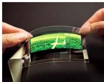
Figura 3.5-3 Display OLED flexible
