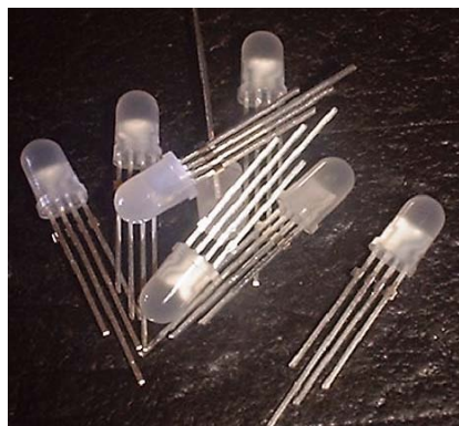
Figura 3.3-5 LED RGB de quatre terminals
