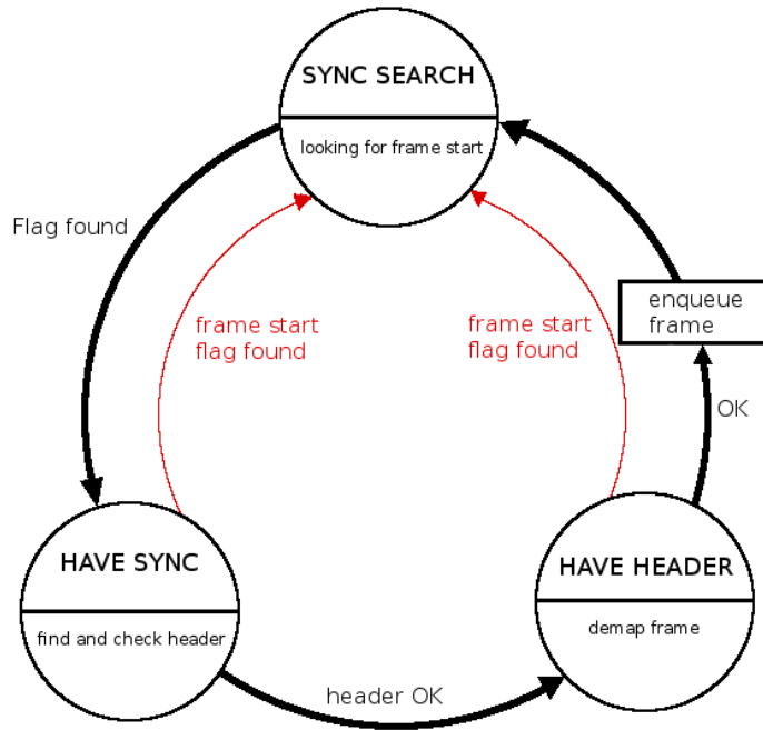
Figure 4.3: Block representation of the state machine in the frame_sink module
