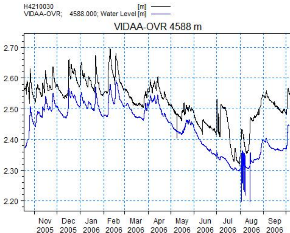
Figure 28 - Water levels comparison between Observed and Simulated data in the Up Stream (Tonder)
