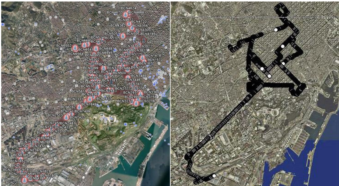
Figure 4.1 In the left Screenshot there are the original WGS coordinates taken with Google earth and in the right we can observe the processed ED50 Spindle 31 coordinates.
