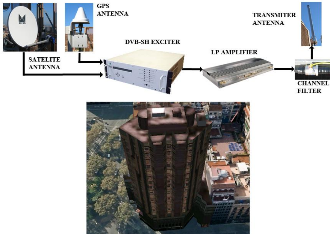
Figure 3.3 Equipment installed in Urquinaona site
