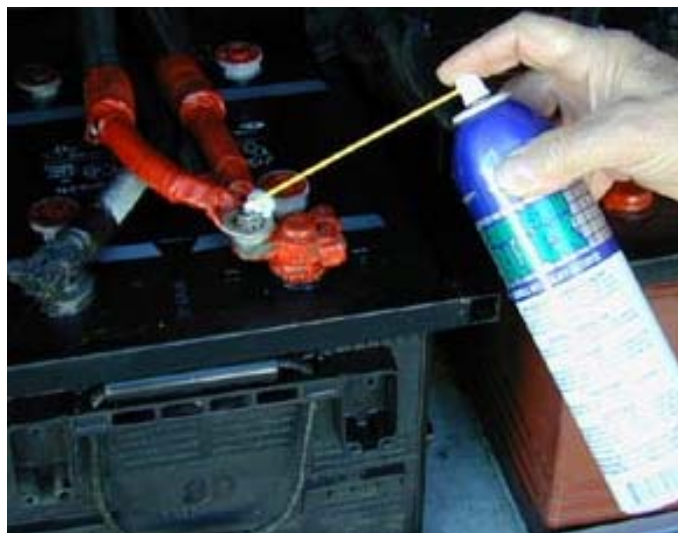
Figure 2-4: Plastic sprayed on to the external parts of the battery
