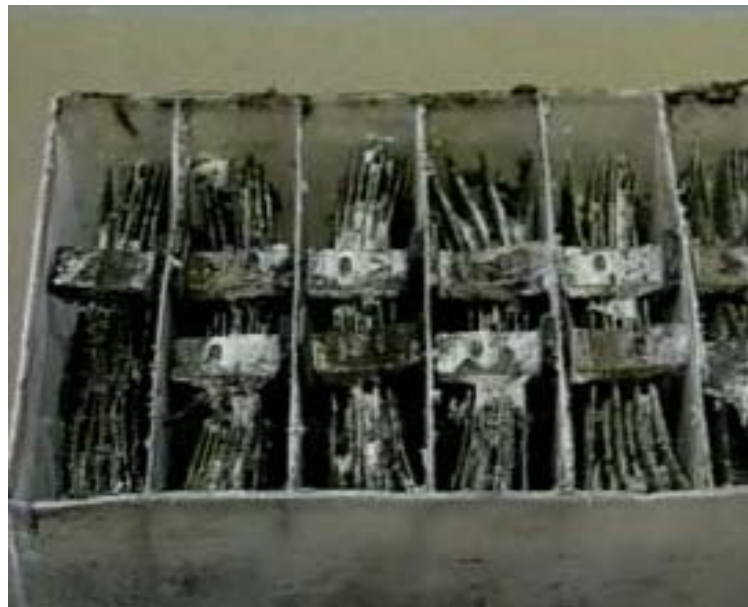
Figure 2-5: Sulfation inside the battery
