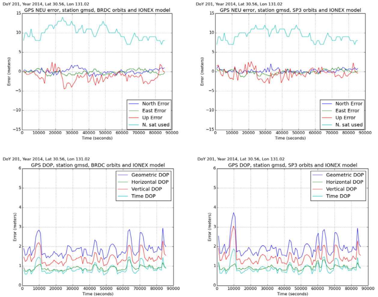
Figure 8.18 NEU error and DOP of GPS with IONEX model At GMSD station (Up Left: NEU errors with broadcast file; Up Right: NEU errors with SP3 file) Down Left: DOP with broadcast file; Down Right: DOP with SP3 file)
