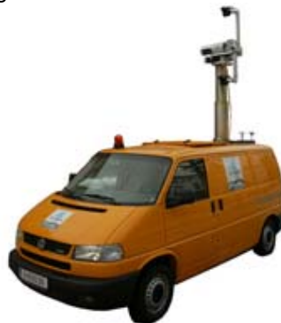
Figure 10: Multi-sensor system for façade documentation.
