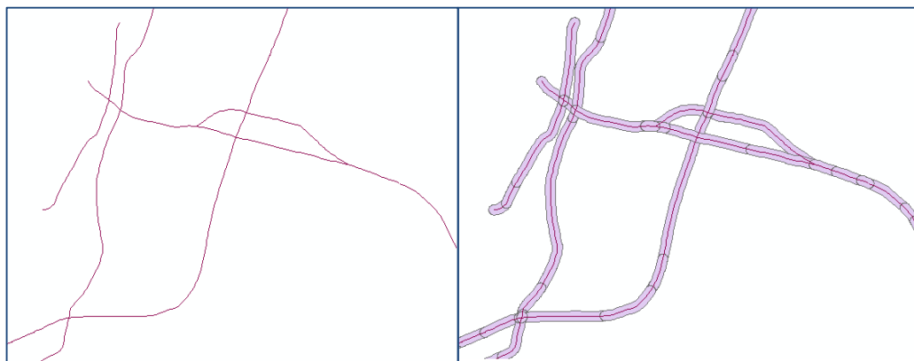
Figure 4.21: Primary Roads Before and After Buffer Placement
