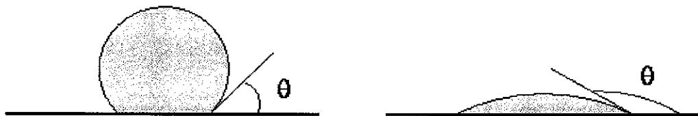
Figure 2.3: A liquid droplet in equilibrium with a horizontal surface surrounded by a gas. The wetting angle ' \theta ' between the horizontal layer and the droplet interface defines the wettability of the liquid. To the left: A non-wetting fluid with 0^\circ \leq \theta \leq 90^\circ . To the right: A wetting fluid with 90^\circ \leq \theta \leq 180^\circ [56].
