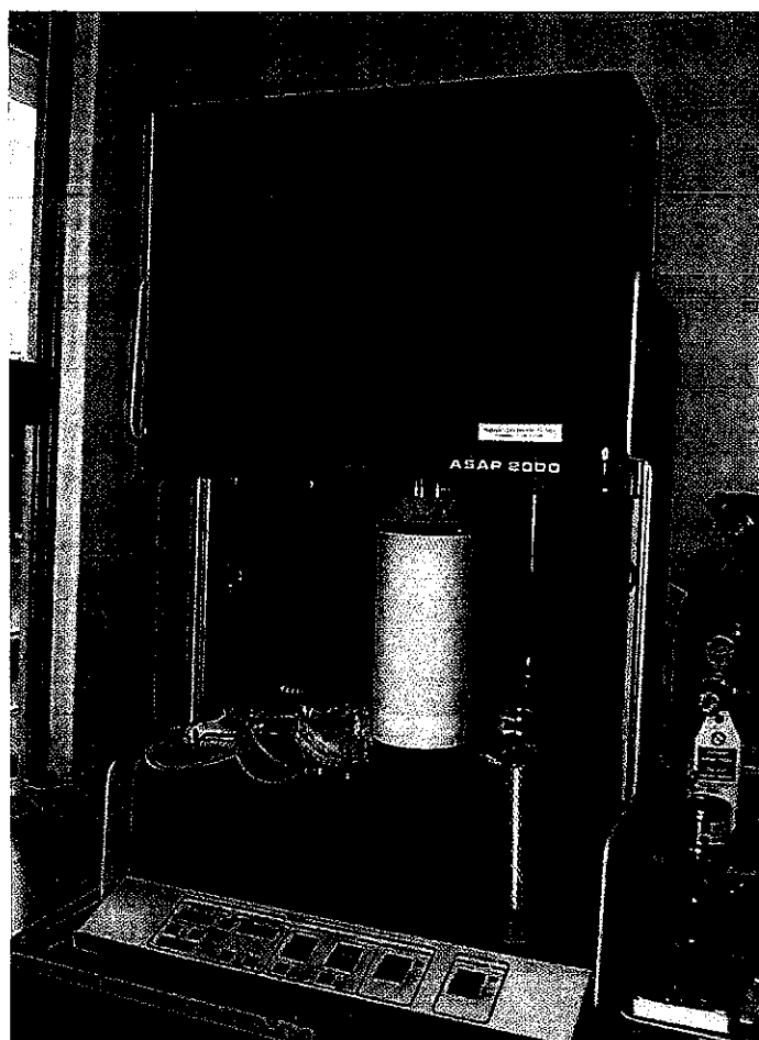
Figure 3.25: Micrometrics ASAP 2000 surface area and pore size analyzer.
