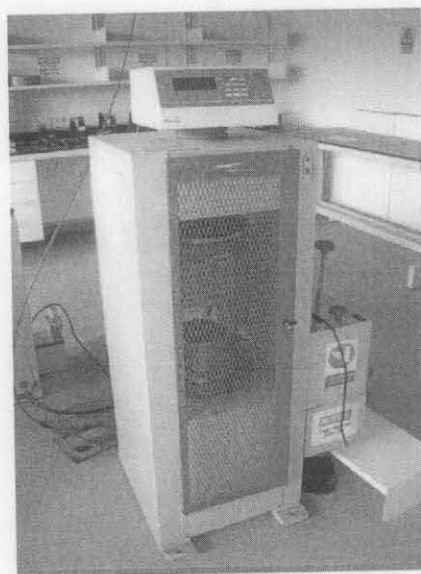
Figure 3. 12. Compression Machine (ELE ADR 3000)
