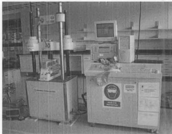
Figure 3. 13. Test setup profile for Flexural strength test
