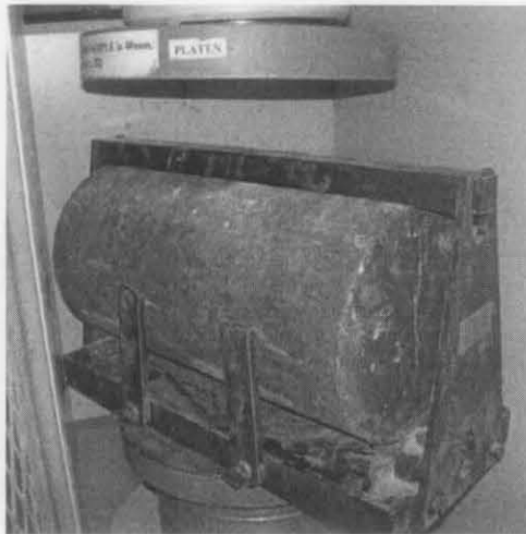
Figure 3. 14. Test setup profile split cylinder test
