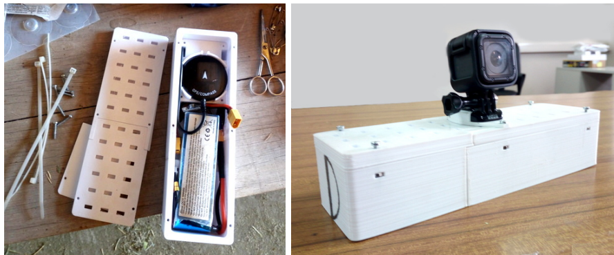
Fig. 1. Data acquisition system with video camera.
