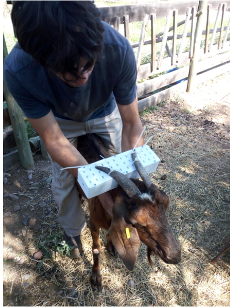
Fig. 2. Data acquisition system placed on the head of the goat.
