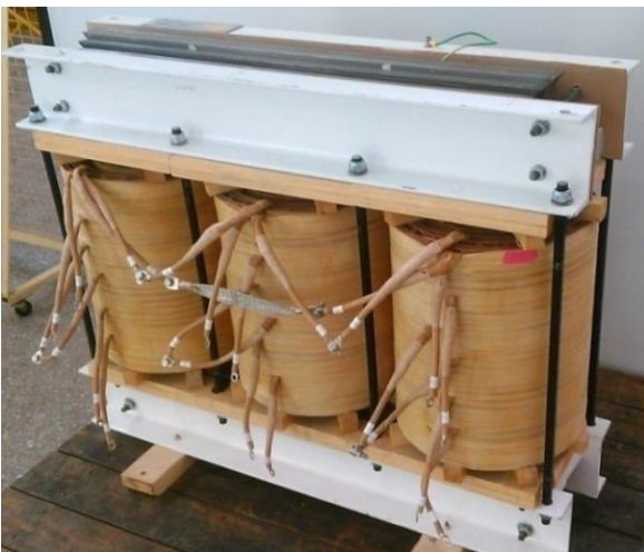
Fig. 5. Transformer used to emulate mechanical defects
