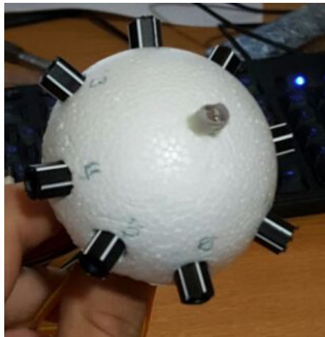
Fig. 3. The semi-sphere shape sensor showing the position of the LDRs.
