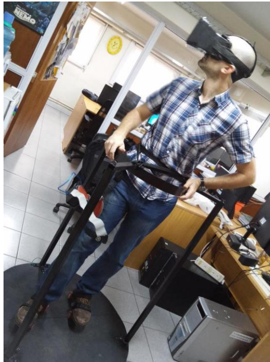
Fig. 2. User on the omnidirectional platform. He is wearing a HMD running a Unity3d application on an Android tablet, and the Arduino Module is attached to his leg.
