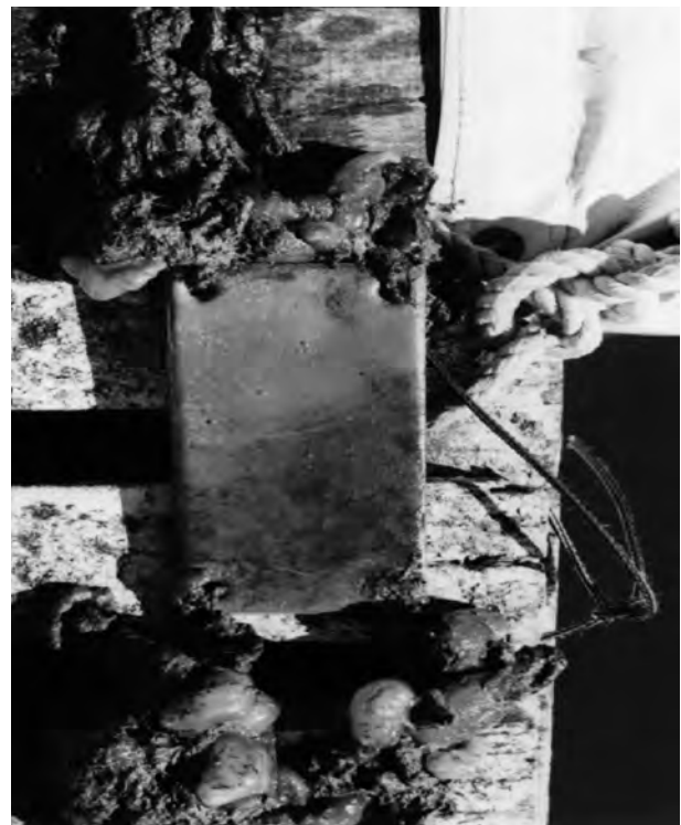
Figure 7. Panel covered by saturated copper coating (B) after six month of immersion.
