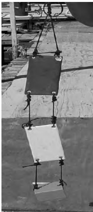
Figure 2. General view of the series of panels before immersion. Top, panel covered by saturated copper coating (B); Bottom, control panel (without copper).
