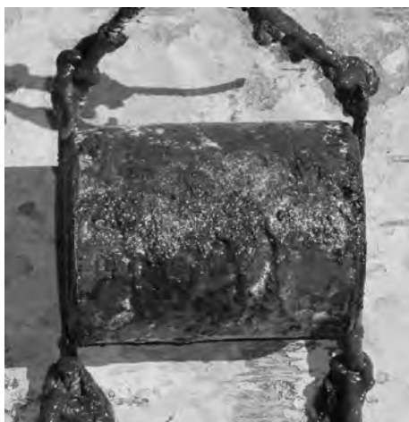
Figure 3. Pipe covered by saturated copper coating (A), after six month of immersion.
