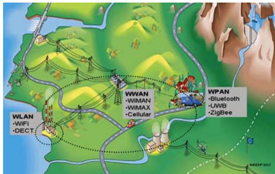
Fig. 5. Wireless technologies for utilities applications
