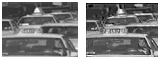
Figure 12. Bicubic interpolation vs. Super Resolution technique by POCS
